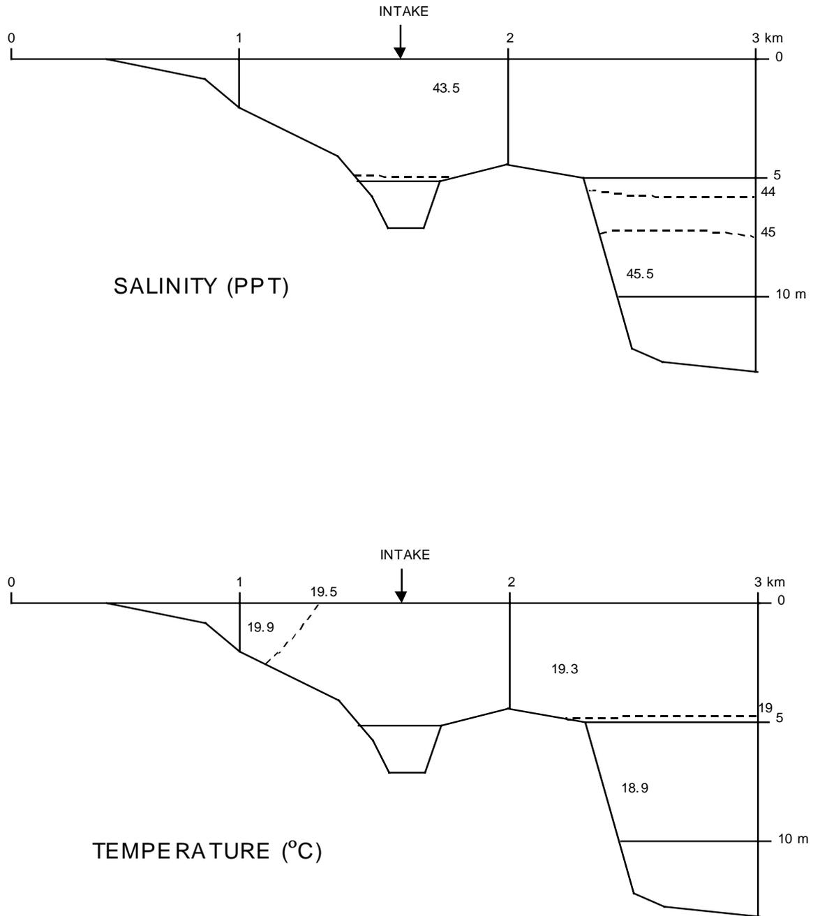
Note: Sections are vertical, along the intake axis (in direction due east), and are measured from the centerline of the site co-ordinate system.
