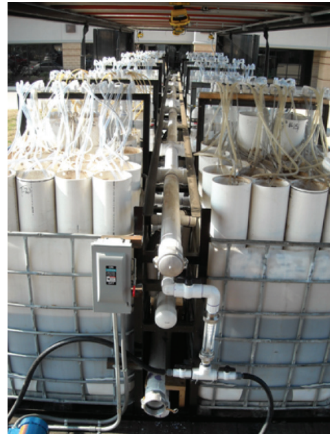
Figure 20: Mobile fracture water preparation / flow back water concentration unit. Taken from [47]
